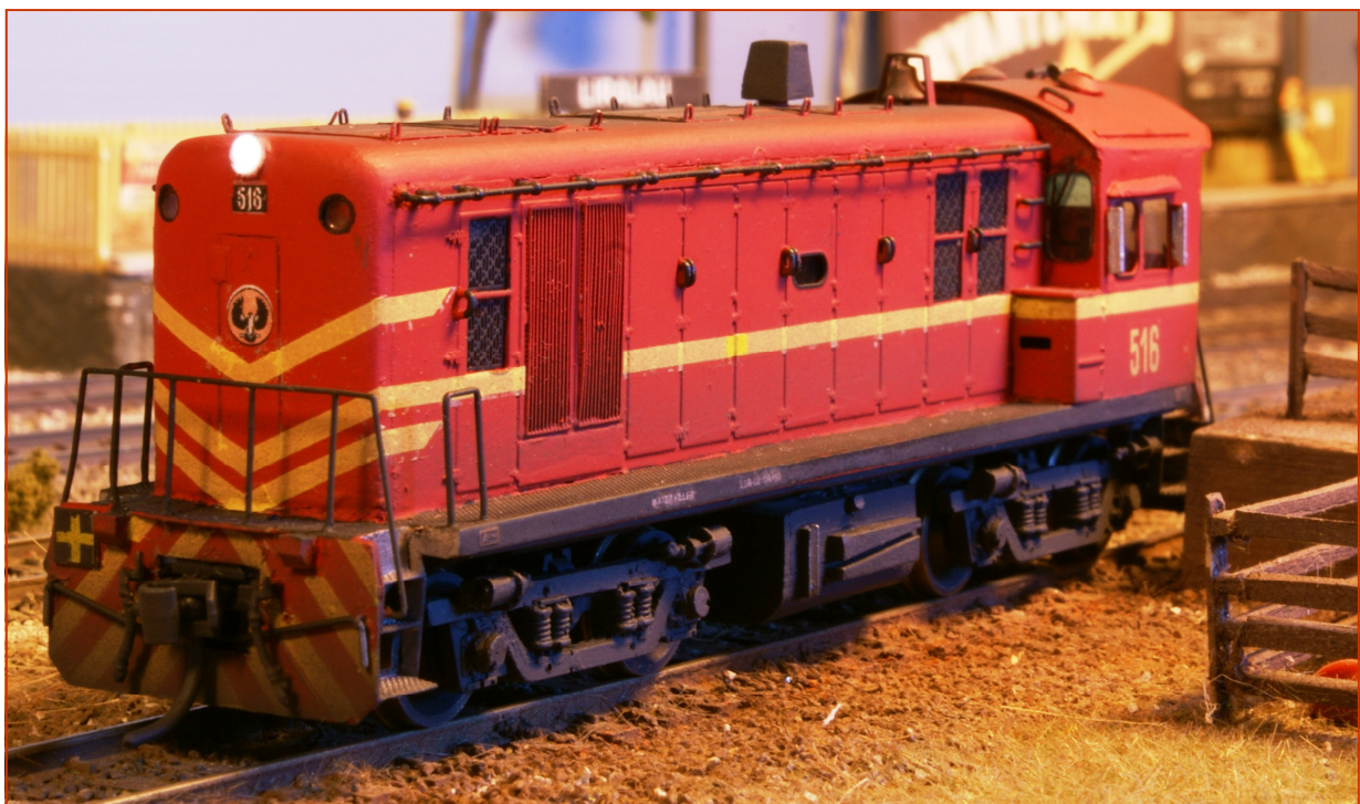
The completed model with replacement side frames
